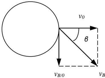
$$\overline{v_B} = \overline{\omega} \times \overline{r_{B/O}} + \overline{v_O}$$
