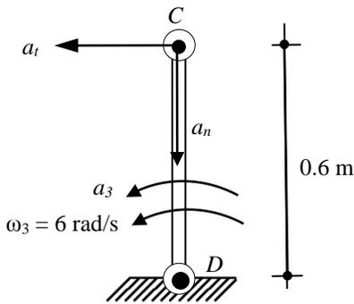
$$\begin{aligned}\overline{a_C} &= \overline{\alpha_3} \times \overline{r_3} - \omega_3^2 \overline{r_3} \\ \overline{a_C} &= \alpha_3 k \times 0.6j - 6^2(0.6j) \\ \overline{a_C} &= -0.6\alpha_3 i - 21.6j\end{aligned}$$
